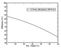
The efficiency curve of the solar collector at the volume flow of 4.3 l/min is:
