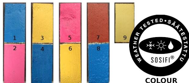
**Fig. 1.** Samples under test, photographed before the exposure. The test samples were 9 paints, painted on boards. The size of a board was 29.7 cm × 7.0 cm × 2.2 cm.
